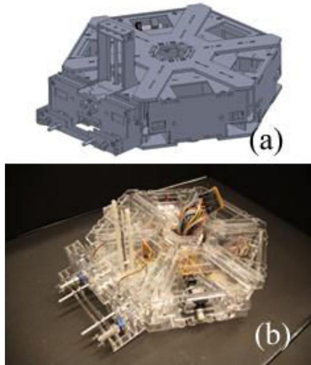
Figure 1. The Hex-DMR System: CAD model (a) and physical implementation (b).
