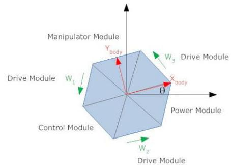
Figure 6. Hex coordinate frames in relation to module position.
