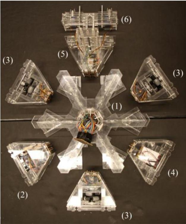
Figure 2. The modules of the Hex-DMR system represented in exploded view
