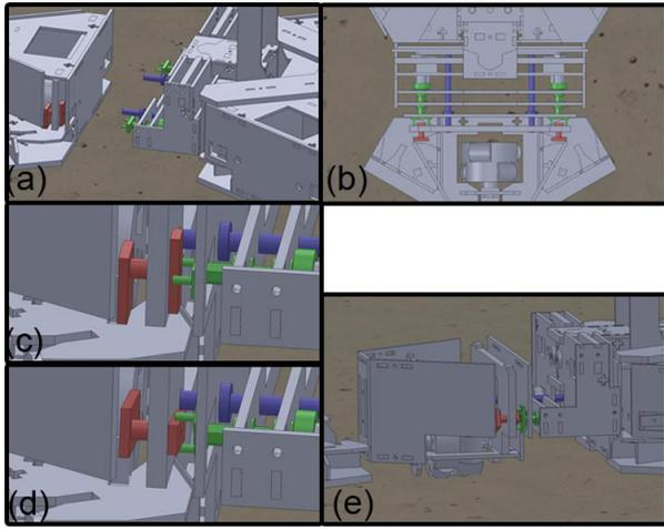
Figure 3. Module latching procedure
