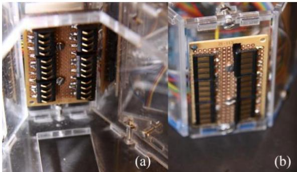
Figure 4. The male, frame mounted (a) and female, module mounted (b) connectors.
