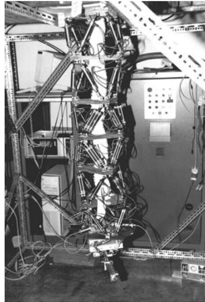
Fig. 2. An Example D-ARM (6 × 6-bit 3D Binary Parallel/Serial Hybrid Arm)
