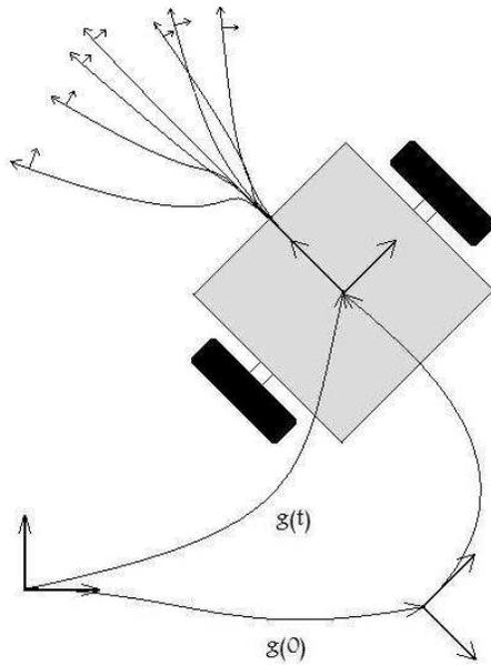
**Fig. 2.1.** A Kinematic Cart with an Uncertain Future Position and Orientation
