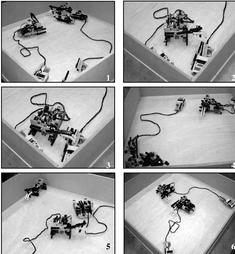
Figure 9: The Self-Replicating Process of the Robot 4.
