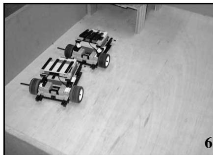
Figure 3: The Self-Replicating Process of the Robot 1.
