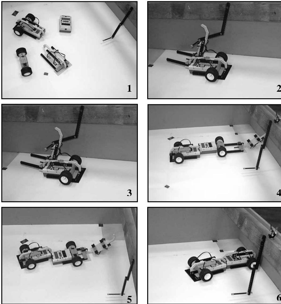
Figure 7: The Self-Replicating Process of the Robot 3.
