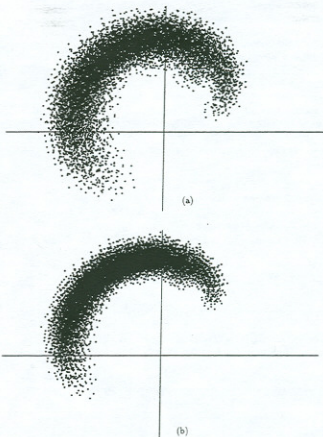
Fig. 2 Workspace of 15-bit manipulator with: (a) (q_i^{\min}, q_i^{\max}) = (3/20, 5/20) (b) (q_i^{\min}, q_i^{\max}) = (4/25, 6/25) ; for i = 1, \dots, 15
