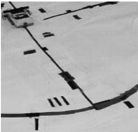
Fig. 1. Barcode scheme used inside the main track
