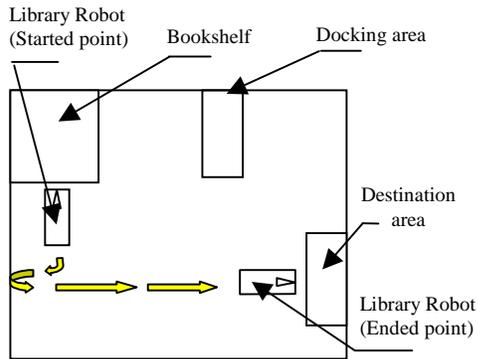
Figure 7 (b): Robot motion planning of the path section 2.
