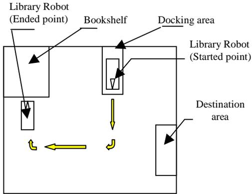
Figure 7 (a): Robot motion planning of the path section 1.
