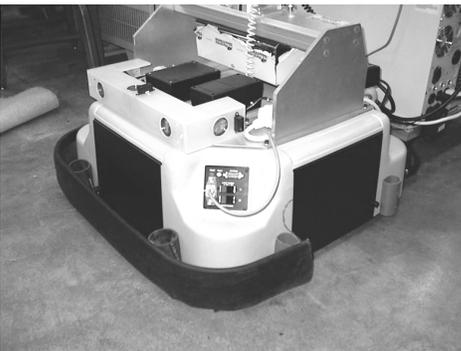
Figure 4: The sensor module.
