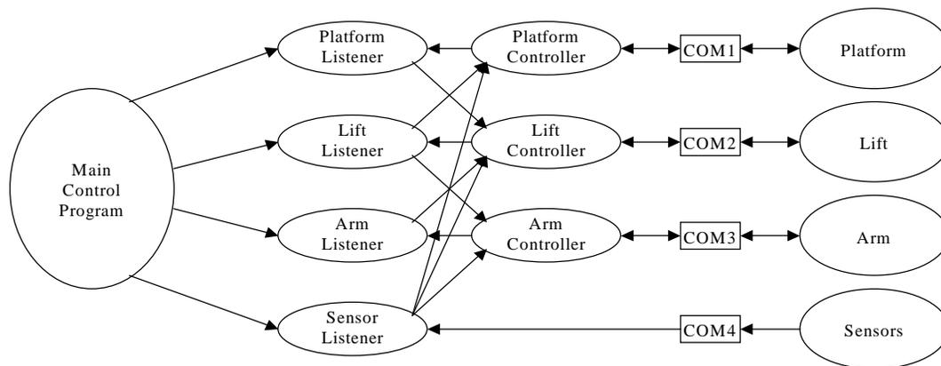
Figure 5: Software structure of the library robot.
