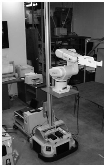
Figure 1: The vertical translation system integrated with the robot manipulator.
