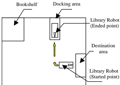
Figure 7 (c): Robot motion planning of the path section 3.
