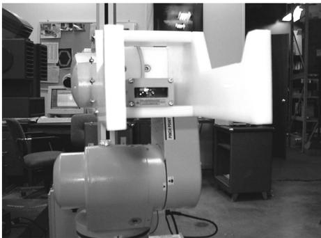
Figure 2: The gripper with a built-in barcode scanner.
