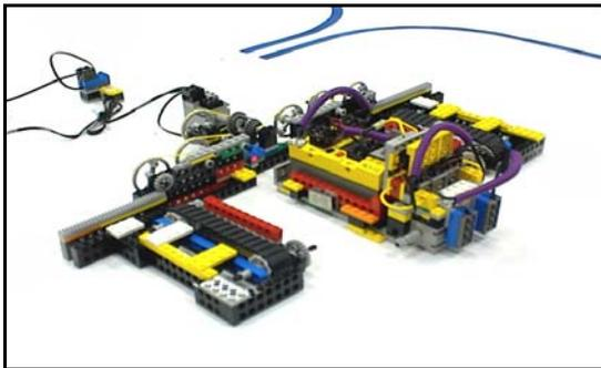
Figure 7: Activation of station 2 when the chassis triggers the station's light sensor.
