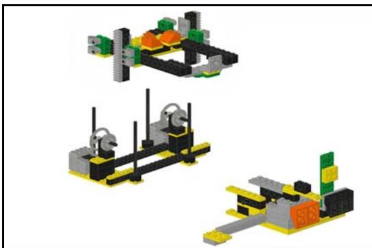
Figure 8: An exploded view of station 3 and the gripper unit.
