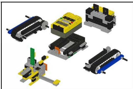
Figure 2: An exploded view of Robot1.
