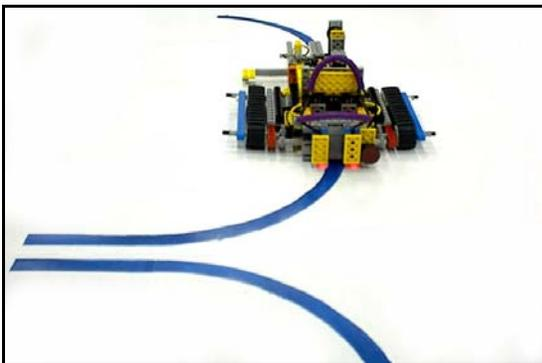
Figure 3: Robot1 autonomously tracking a painted line with the light sensors.
