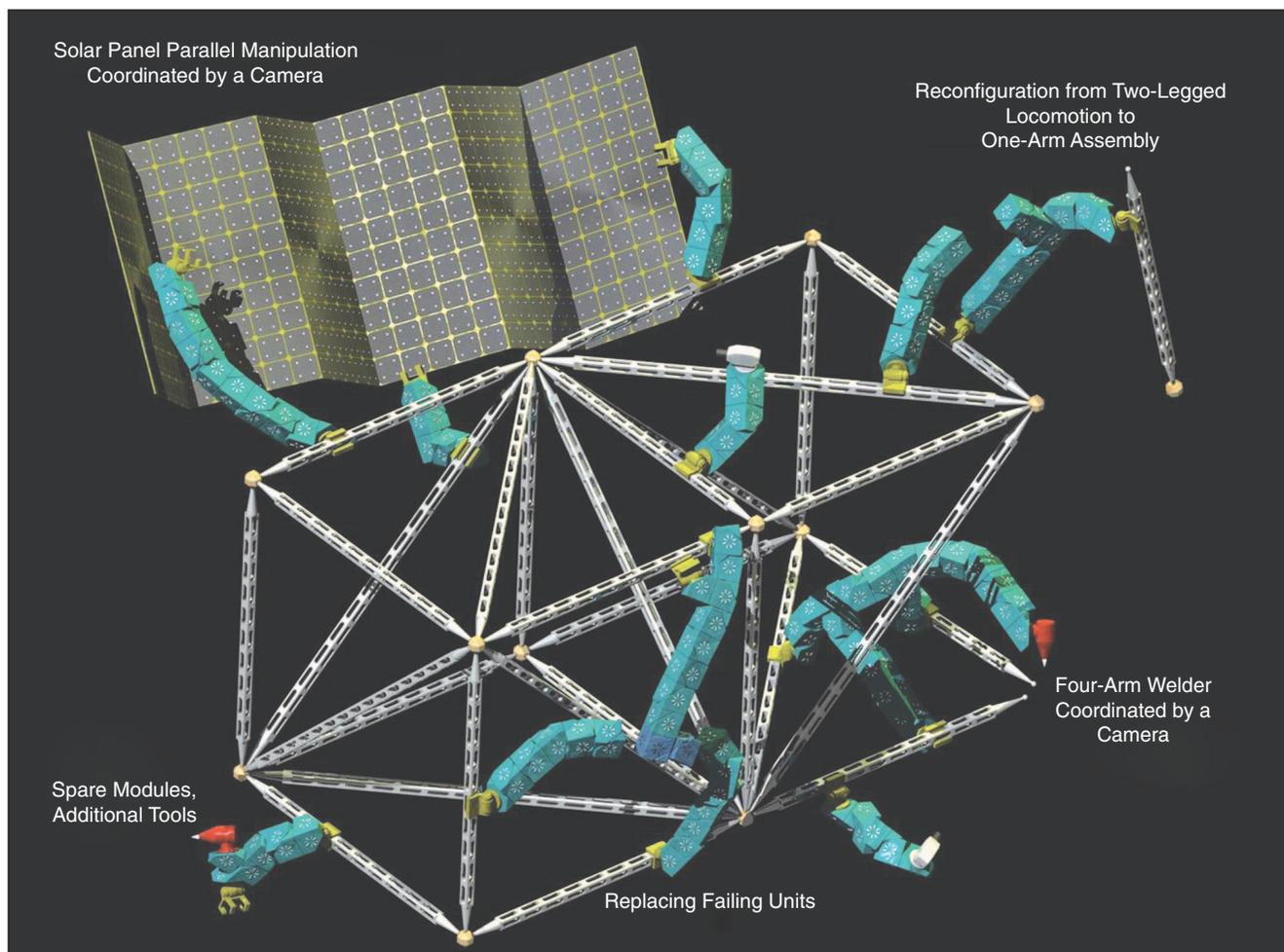
**Figure 1.** Artist rendition of a space application of modular robotics, showing a truss-building colony of chain/tree robots composed of cubical modules, configured in various morphologies for a variety of tasks including assembly, cooperative manipulation, and self-repair (from [1]).
