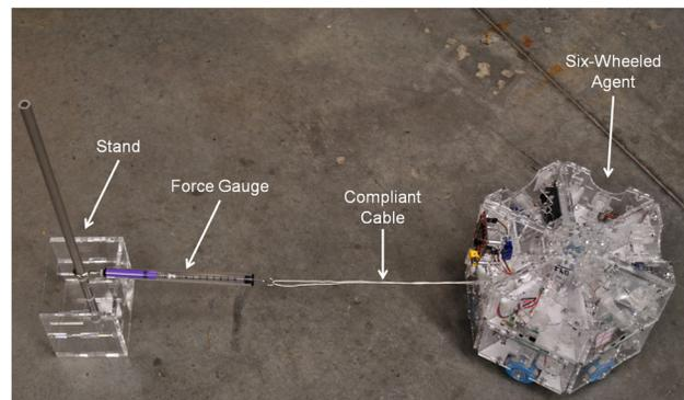
**Fig. 15 Experimental setup for measuring the maximum tractive force on concrete**
